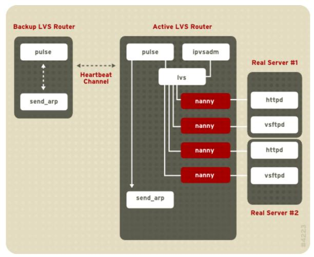
Figure 1.5. Load Balancer Add-On Components
